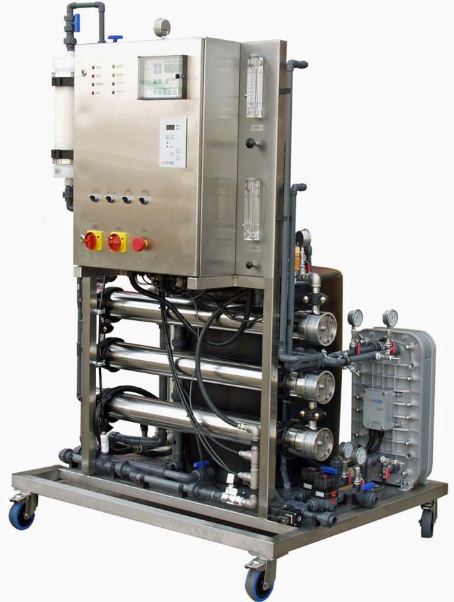
Reverse osmosis is therefore considered a much safer route of producing pure water for many commercial and industrial applications, and additionally the plant doesn't need to be taken out of service for regeneration as a demin plant does.
